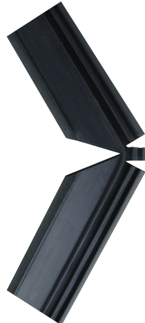
Notching a frame corner - Y-cut
